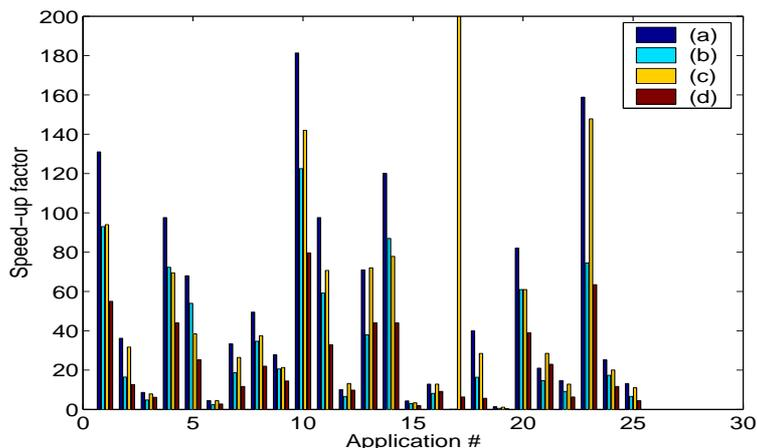
Figure 1: `slmoen4` with fast QR versus MATLAB 6.5.1 `n4sid` with QR factorization and default options, but `order = n`, `'N4Weight' = 'MOESP'`, and: (a) `'Cov' := 'CovarianceMatrix' = [ ]`, `'N4H' := 'N4Horizon' = 'Auto'`; (b) `'Cov' = 'None'`, `'N4H' = 'Auto'`; (c) `'Cov' = [ ]`, `'N4H' = [ s s s ]`; (d) `'Cov' = 'None'`, `'N4H' = [ s s s ]`, see also [31].
