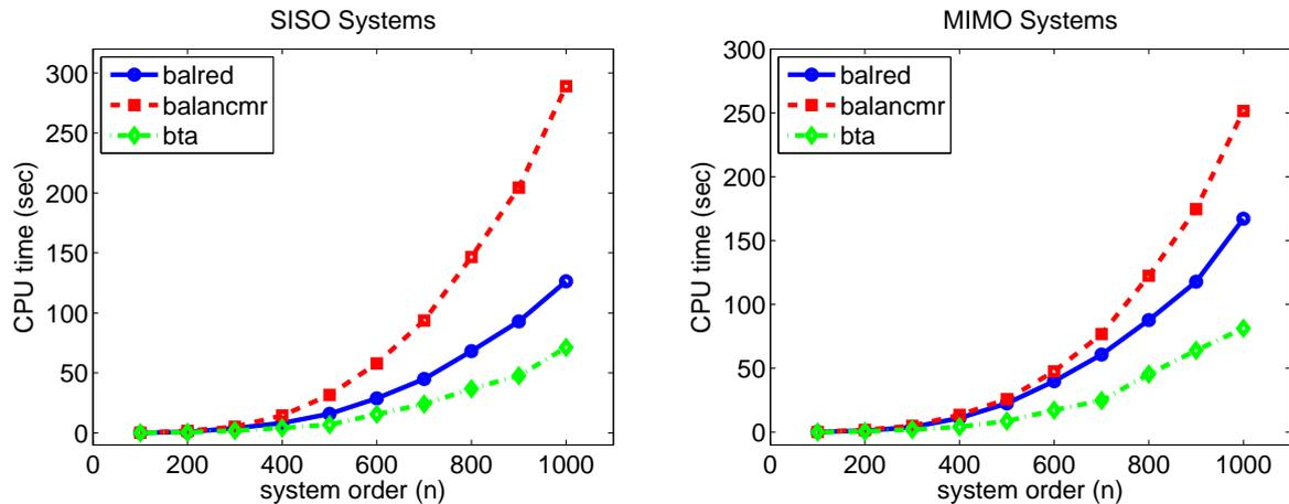
Figure 2: Comparison of MATLAB functions for balanced truncation for SISO systems (left) and MIMO (right,  $m = p = 10$ ) systems.
