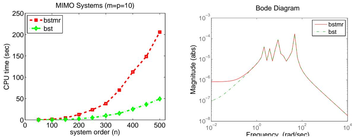
Figure 3: Comparison of MATLAB functions for balanced stochastic truncation: timings (left) and accuracy (right).
